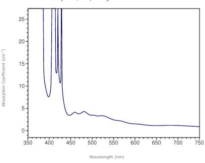
**Transmission absorption spectra** in the UV to near-IR range (250-1000 nm) were collected using a Hitachi U4001 spectrometer (2.0 nm slit, 1.0 nm data interval, and 120 nm/min scan speed). Unless otherwise noted, an unpolarized light beam was focused on the culet area of the optically unoriented sample.
