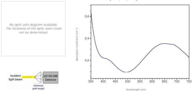
Visible Absorption | min. path length: 9.0 mm
